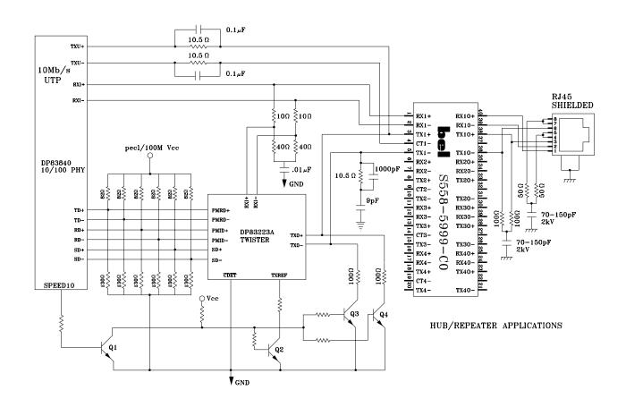
**NOTE:** It is recommended for the above application to leave the secondary side center taps unconnected. For applications with other IC's, please consult the factory for recommendations on center tap termination and layout schematic.
